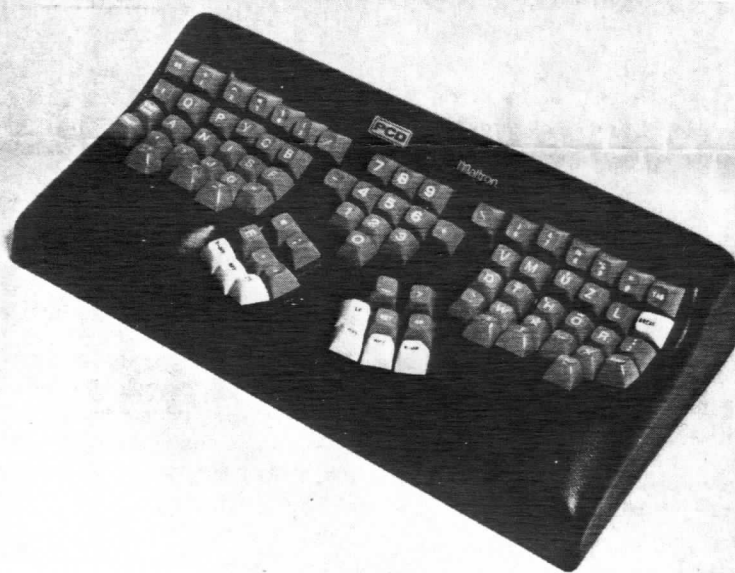
Maltron keyboard for computer terminal with central number group and cursor control keys on right-hand letters, U up, K down, T left, H home, and O right. These are accessed in the shift and control condition, thus avoiding the need to move the hand to another group.
